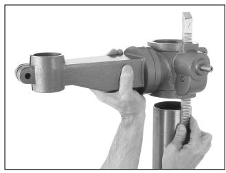
Figure 9. Sliding table support and rack over the column.
